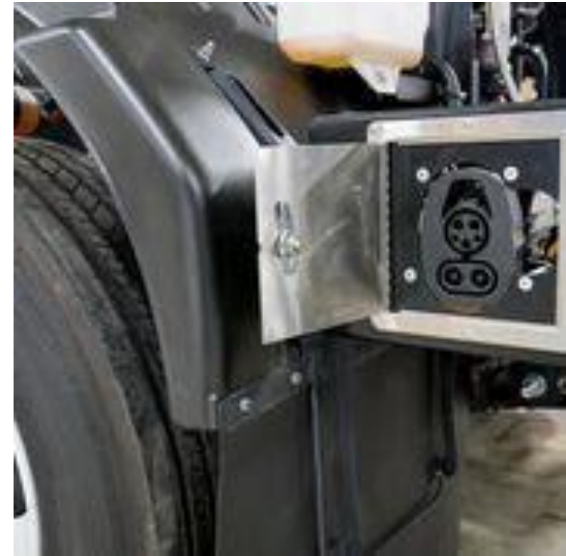
The DC Fast Charge port, SAE J1772 CCS Combo Type 1
