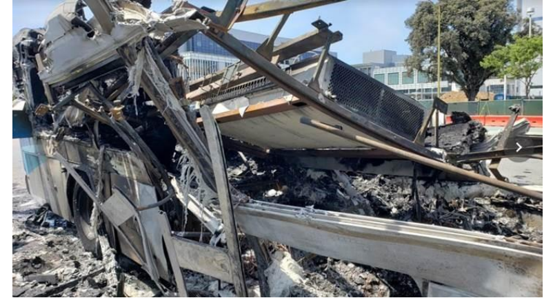
An Electric Scooter Taken On Board the Bus Caught Fire and Spread to the Rest of the Bus. The Bus Hybrid Electric Battery was Intact After the Fire
