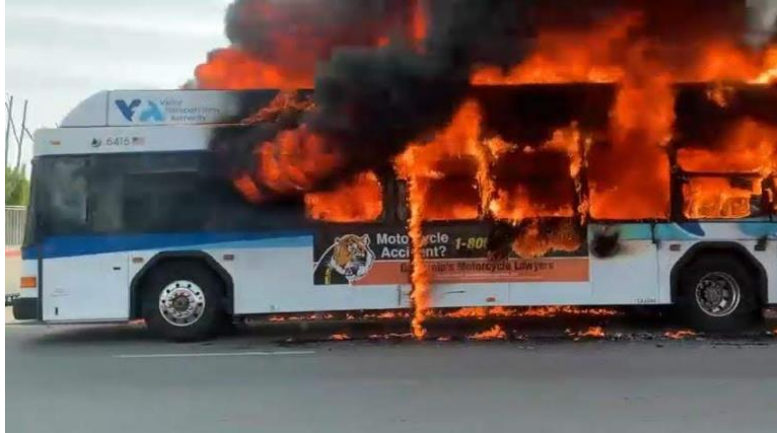
An Electric Scooter Taken On Board the Bus Caught Fire and Spread to the Rest of the Bus. The Bus Hybrid Electric Battery was Intact After the Fire
