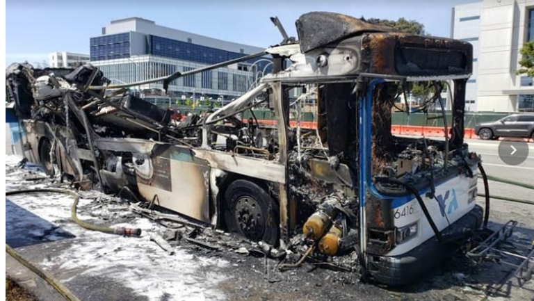
An Electric Scooter Taken On Board the Bus Caught Fire and Spread to the Rest of the Bus. The Bus Hybrid Electric Battery was Intact After the Fire
