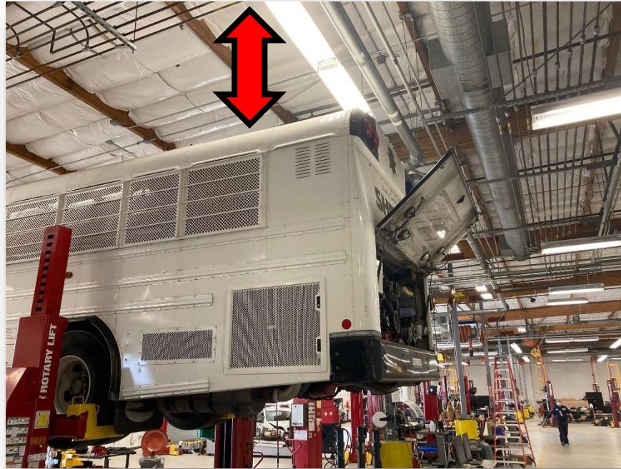
Maintenance Facility - Vehicle to Roof Clearance Sufficient?
